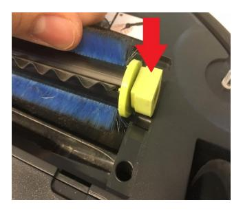
Put the green support assy into the right position (notch into direction brush and round side down) and press it into the holder.
