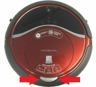
Press the "Push" button in the back to open the dust bin cover.
