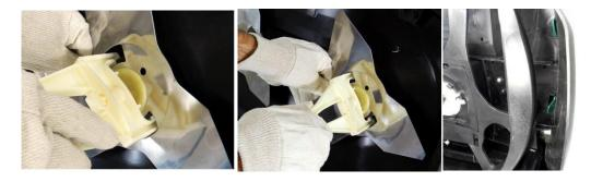
Remove the knife from the Robomow and remove the robomows top cover by pushing the green clips on the third Photo
